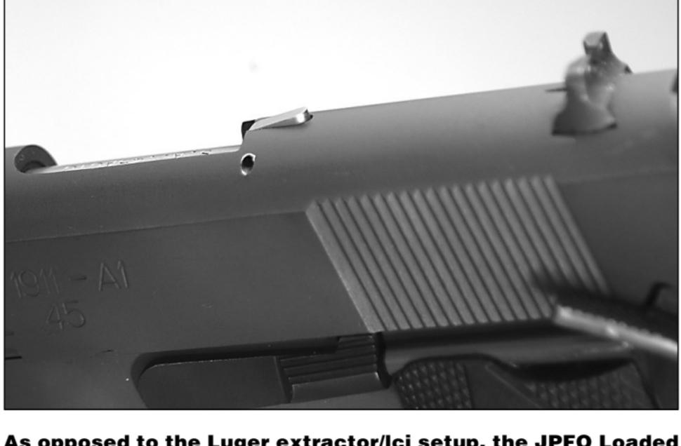
**As opposed to the Luger extractor/LCI setup, the JPFO Loaded Chamber Indicator unit signifies a loaded status by rising at its rear and sloping toward the chamber end of the barrel.**
