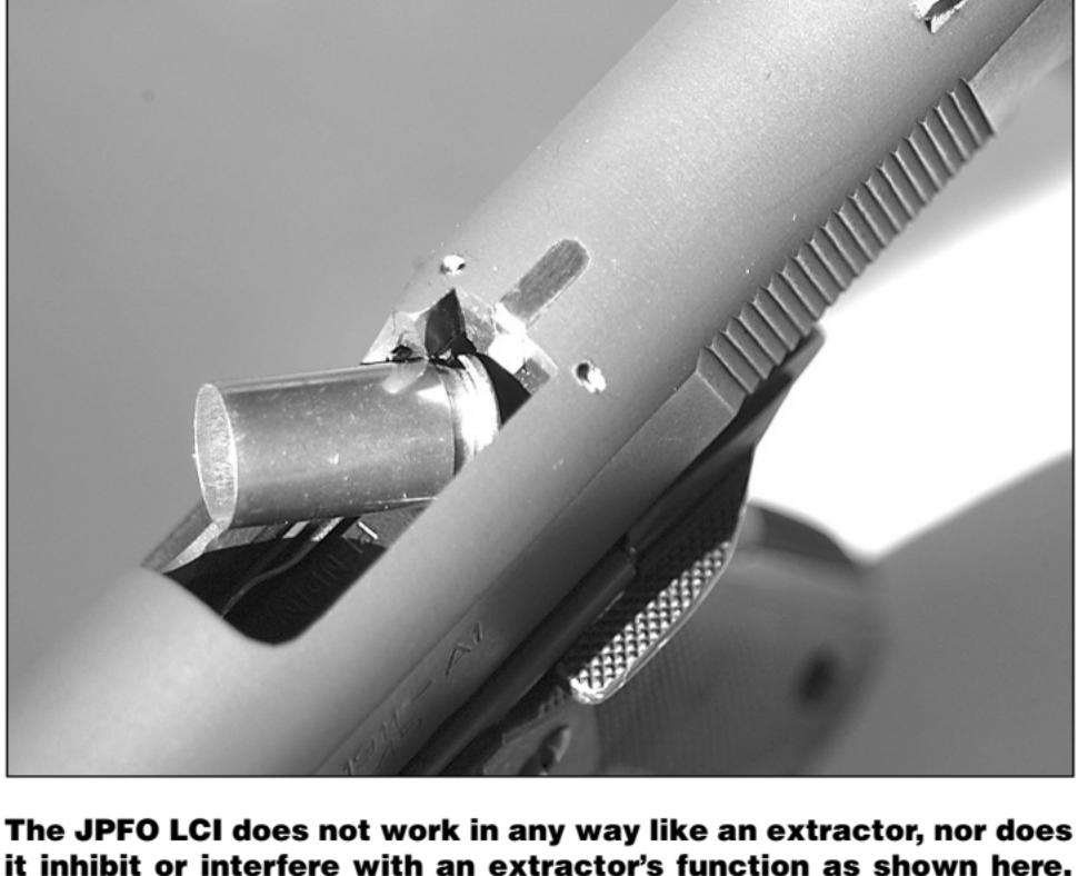
**The JPFO LCI does not work in any way like an extractor, nor does it inhibit or interfere with an extractor's function as shown here. It merely indicates when the chamber of the pistol is loaded.**
