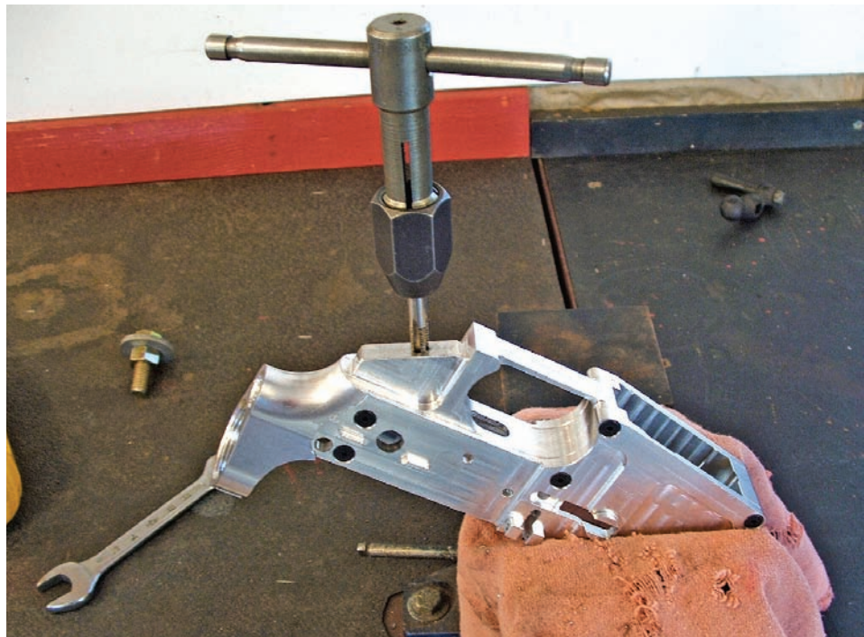
Tapping the larger 1/4" hole is much less stressful than the small, easy-to-break 6/40 tap holes. Even so, use plenty of lube and proper tapping technique here.
