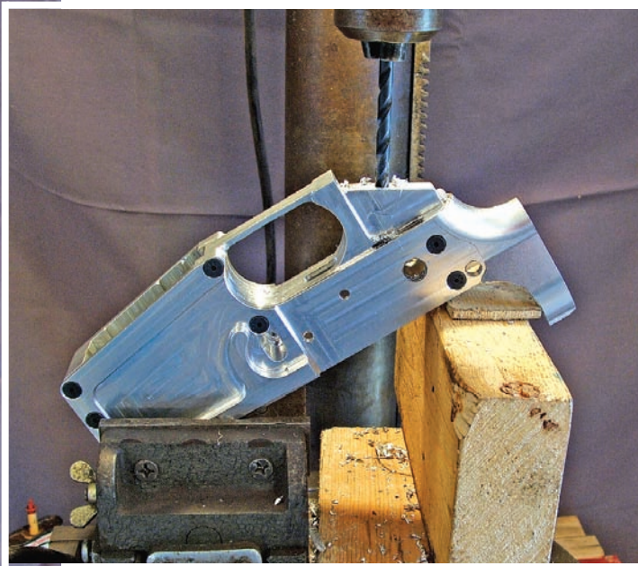
Drilling the takedown pin detent requires good alignment to prevent missing the center of the pin hole. The pistol grip screw has to be drilled at the correct angle.
