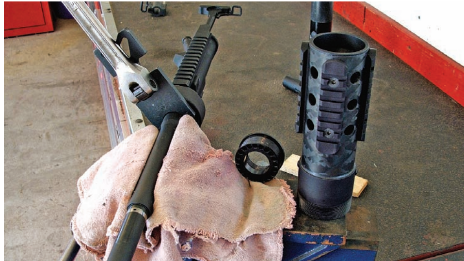
The original barrel nut must be replaced with PRI's special barrel nut to install the carbon fiber handguard. There's no substitute for the right tool here.
