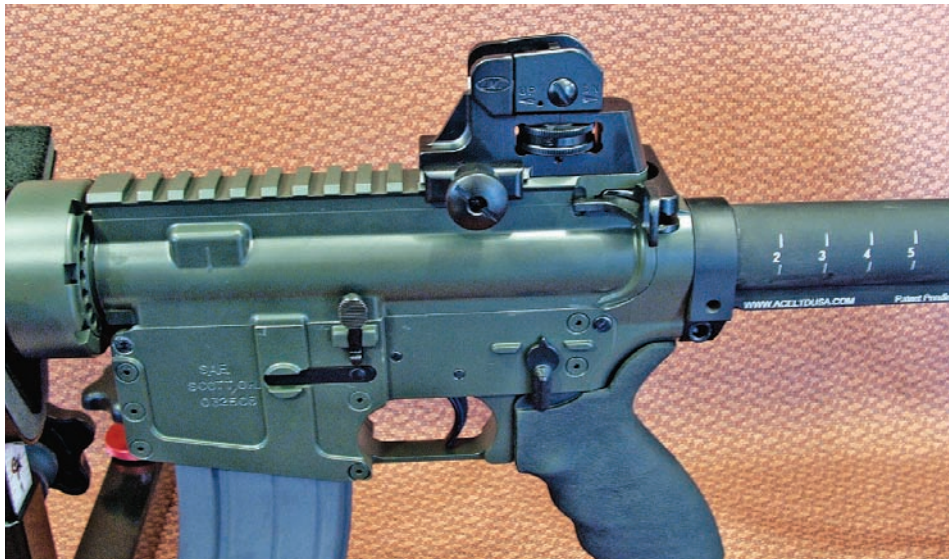
One of the benefits of using a flat-top upper like this Model 1 Sales receiver is its ability to accept various sighting options. You can go optical or conventional.
